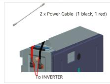
Step6: Connect the power cable from the battery 1 to the inverter.
